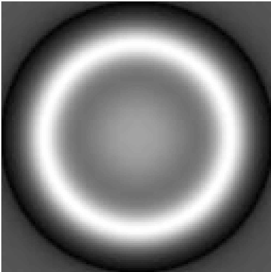
**Figure 3:** Reconstructed cross section of a  $50\ \mu\text{m}$  capillary filled with water. The frequency spectrum was calculated according to the *line shape function* in a  $8\ \text{G}/\text{cm}$  gradient with  $0.4\ \mu\text{m}$  resolution. The length of the frame corresponds to  $50\ \mu\text{m}$ , the diffusion constant is that of water,  $3 \times 10^{-5}\ \text{cm}^2/\text{s}$
