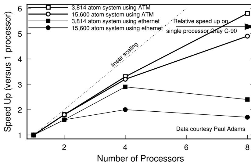
Figure 1: Speedup of Parallel X-PLOR for a simulation of a 3,814 and a 15,600 atom system on the Resource's workstation cluster utilizing the ATM network or the ethernet network. The relative speed for both systems on a single processor Cray C-90 is marked for reference. Data courtesy Paul Adams, Yale University.
