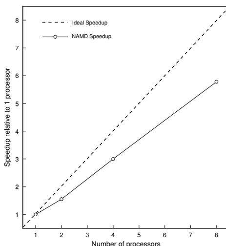
Figure 2: Speedup of **namd** for a simulation of a 10,000 atom system on the cluster of HP workstations within the Resource.
